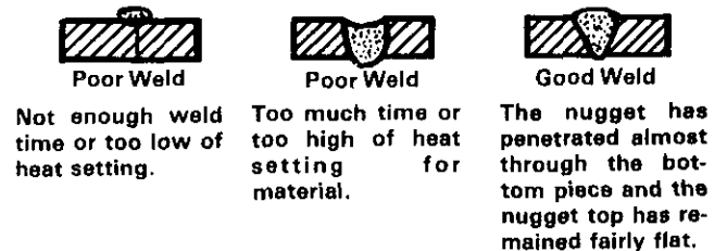
Figure 5-7. Various Spot Welds
