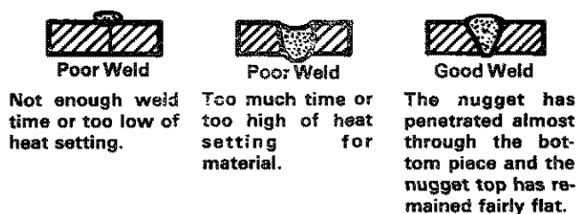
Figure 5-7. Various Spot Welds
