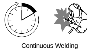
100% Duty Cycle at 120 Amperes DC
