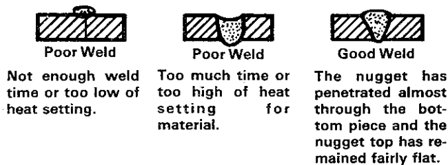
Figure 5-7. Various Spot Welds
