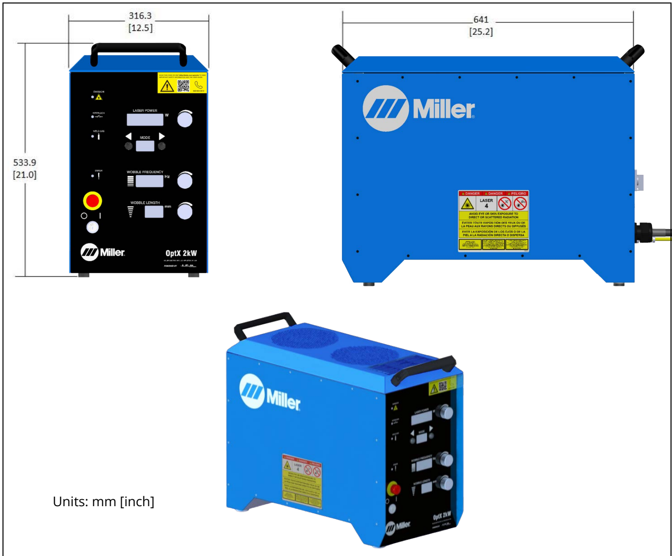
▼ Figure 9. Device Layout and Dimensions
