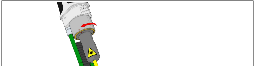
▼ Figure 66. Rotate receiver nut to align red dots
