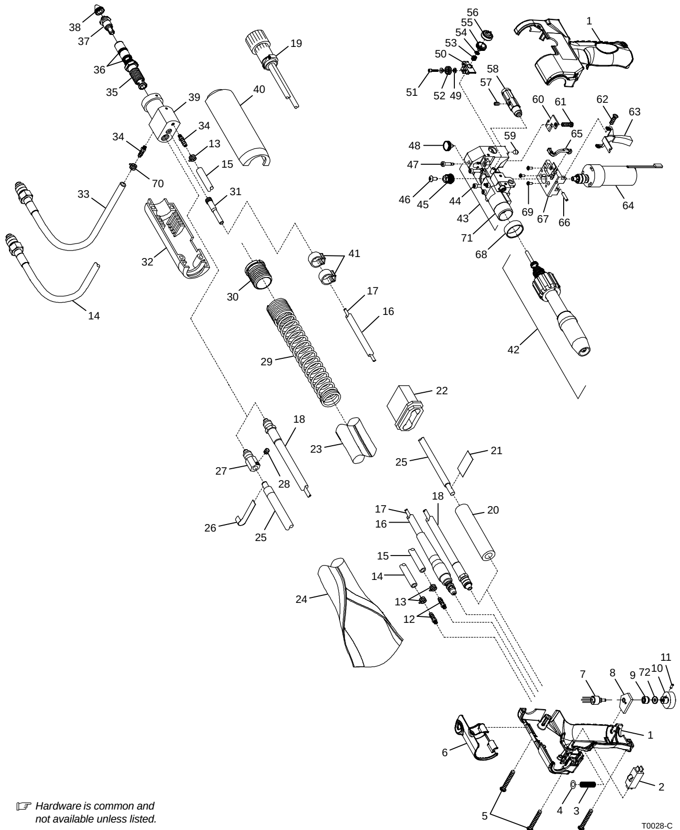
Figure 9-1. Exploded View Of XR - Pistol - Pro Gun
