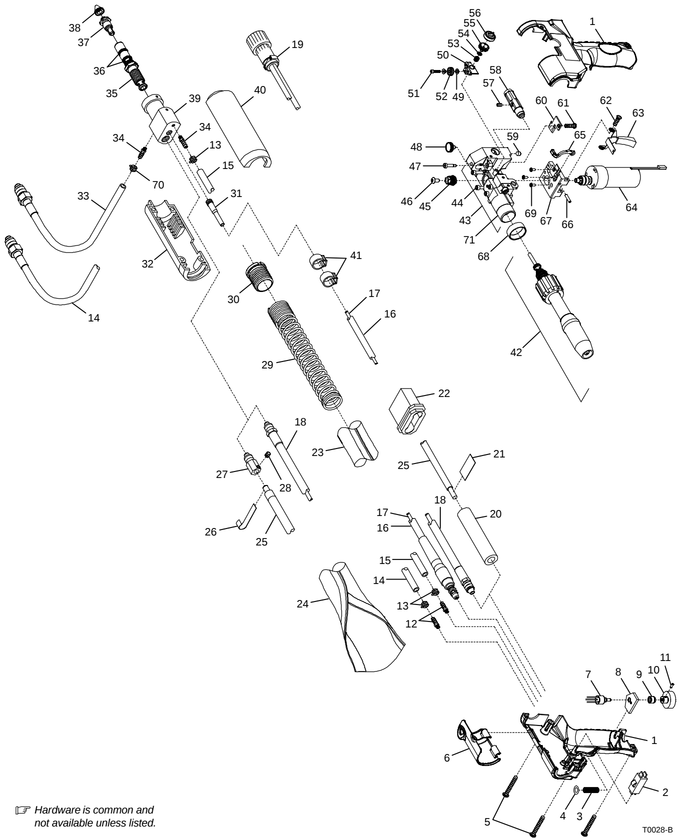
Figure 9-1. Exploded View Of XR - Pistol - Pro Gun
