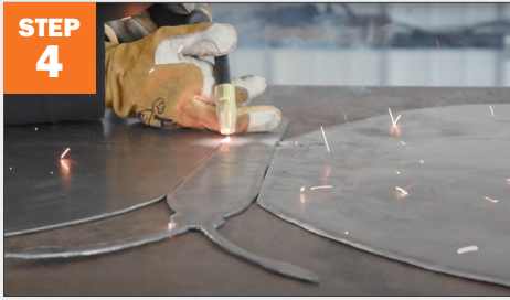
Tack weld the inside of the wings to the body.
