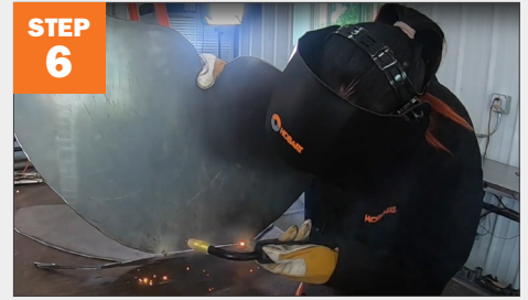
Tack weld the outside of wings to the body.
