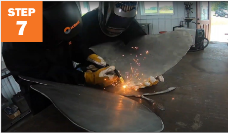
Weld the inside of wings to the body.
