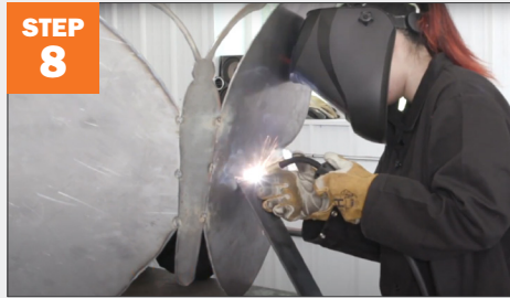
Weld the braces to the back of the wings.
