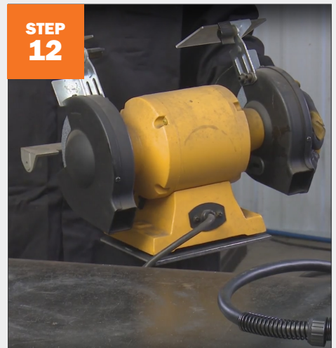
STEP 12 Mount grinder to top plate using the required number of bolts.
