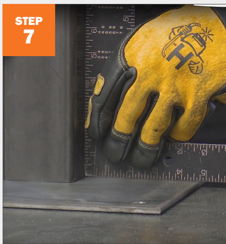
STEP 7 Check to make sure the post is square to the base plate.
